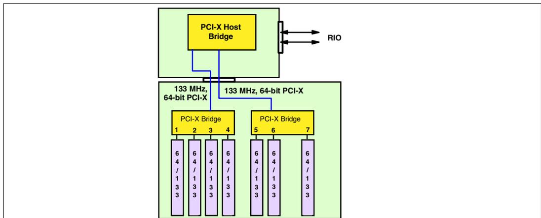
Figure 2-6 Conceptual diagram of the I/O drawer
