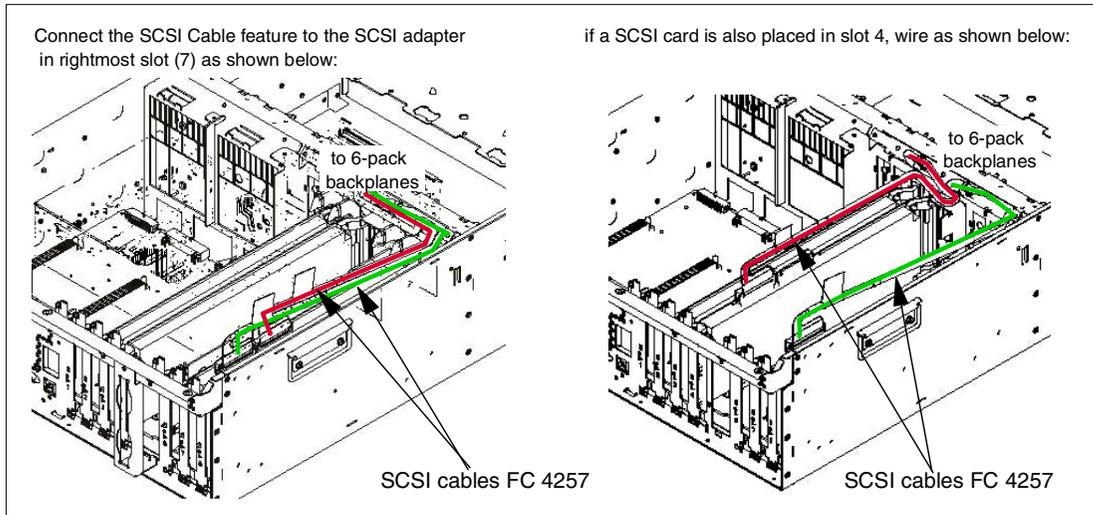
Figure 2-8 Internal SCSI cabling
